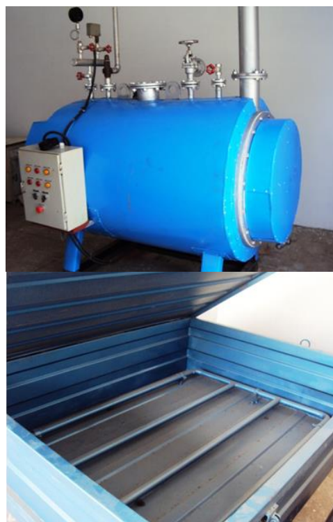
Figure 1. Model steam unit for sterilization of potting media. The steam unit includes a steam generator (left) and a media trolley (right) for sterilization of potting media.
